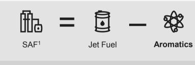
Aromatics cause swelling of nitrile O-rings within fuel system of aircraft and ensure sealing, but also cause increased particulate emissions (less efficient burning)
